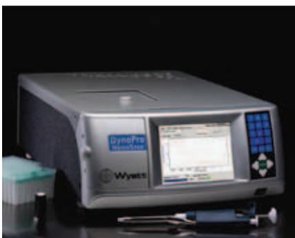
The DynaPro™ NanoStar® can be used for nanoparticle and protein size determination, with sample volumes down to 1  $\mu\text{L}$  and a temperature range from 4-150° C.
